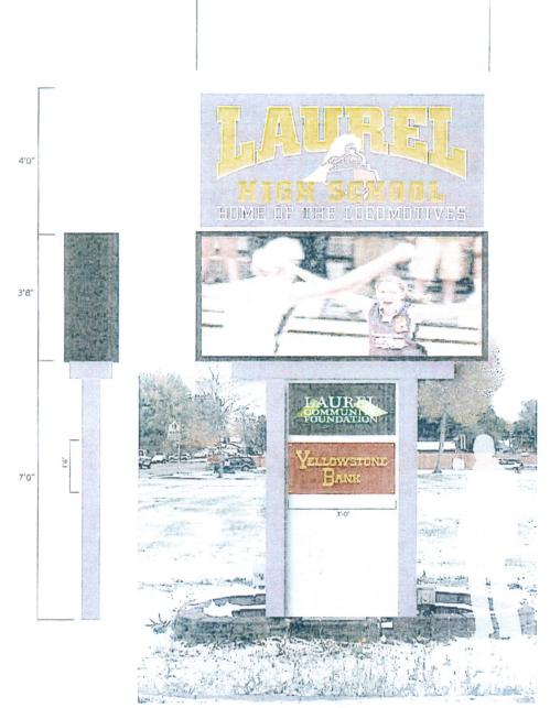
REMODEL EXISTING D/F DISPLAY.REMOVE EXISTING CABINET AND MESSAGE CENTER.NEW FABRICATED GALVANEAL GABINET AND RETAINERS FILMED TUFFAK FACES.ILLUMINATION WHITE LEDS.. NEW GS6 15.85 60X150 RGB MESSAGE CENTER, PAINTED GALVANEAL END FILLERS. 6" PAINTED SQ. TUBE ON EXISTING BOLT BASES.PAINTED ALUMINUM FILLER.FILMED DIBOND SPONSER PANELS.
