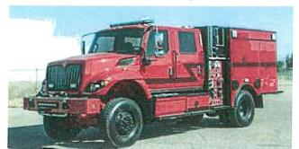
Army 2 ½ ton with a Type 3 or 4 Brush Truck (125-250 gpm pump; 500-750-gallon tank).
