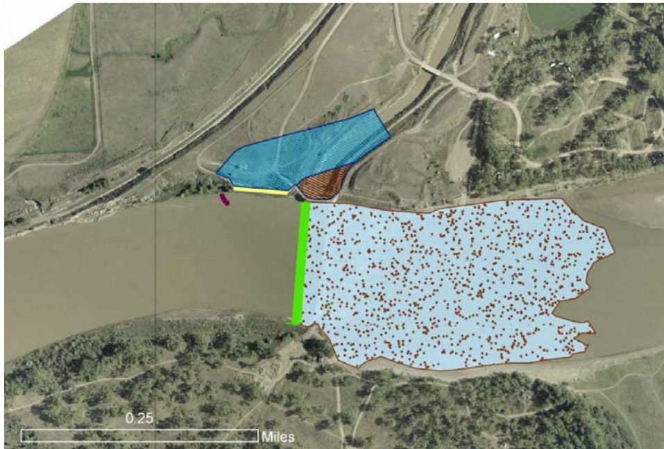
Figure 16: Schematic of preferred alternative for the Intake Diversion Dam. Concrete weir with rock ramp
