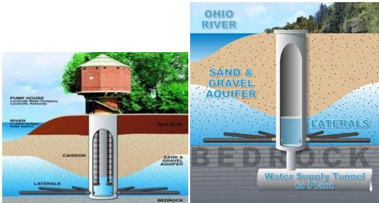
Figure 42: Horizontal collector well
